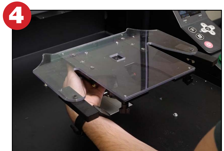
Step 4: Secure the T-Lock Shoe Insert by rotating the center piece in the T-Lock brackets.
