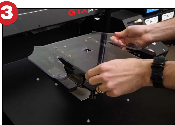
Step 3: Insert the T-Lock Shoe Insert into the T-Lock Base.
