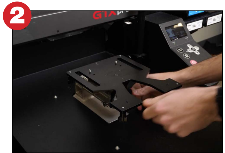
Step 2: Adjust the height of the platen and tighten the locking lever.
