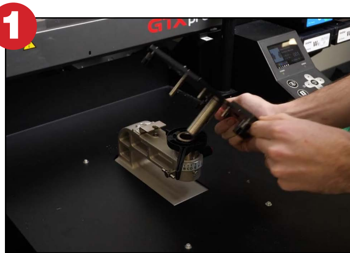
Step 1: Insert the T-Lock Base into the platen stem of the Brother DTG printer.
